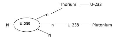
All thermal reactors are example of converters. The spent fuel is processed to get plutonian or U-233
